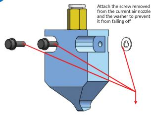
Attach the new air nozzle to the spindle
