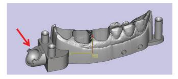
The vertex interface can be placed anywhere on the unit. This means a designer could have the cup <u>higher</u> or <u>lower</u> than the rest of the surface.
