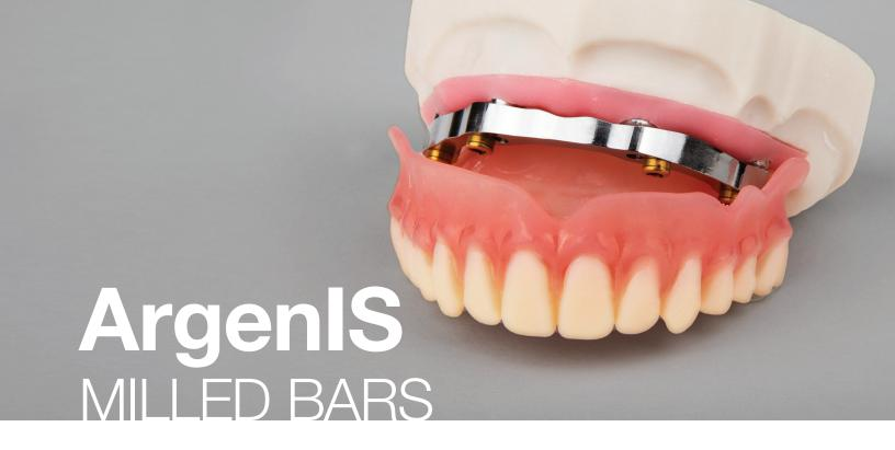
ArgenIS Milled Cobalt-Chrome and Titanium Bars are for use in both fixed and removable cases at the abutment level. These bars are milled from Grade 23 titanium and Argen CoCr 255 with industrial precision 5-axis milling machines. Cobalt-chrome and titanium bars are compatible with most multi-units. Titanium Bars can be received either polished or unpolished. They can also be anodized.
