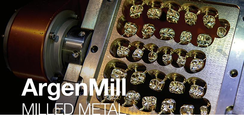
ArgenMill Milled Metal crowns and bridges provide you with a digitally fabricated, accurate representation of a file that offers improved fit and consistency over the traditional wax/cast method.
